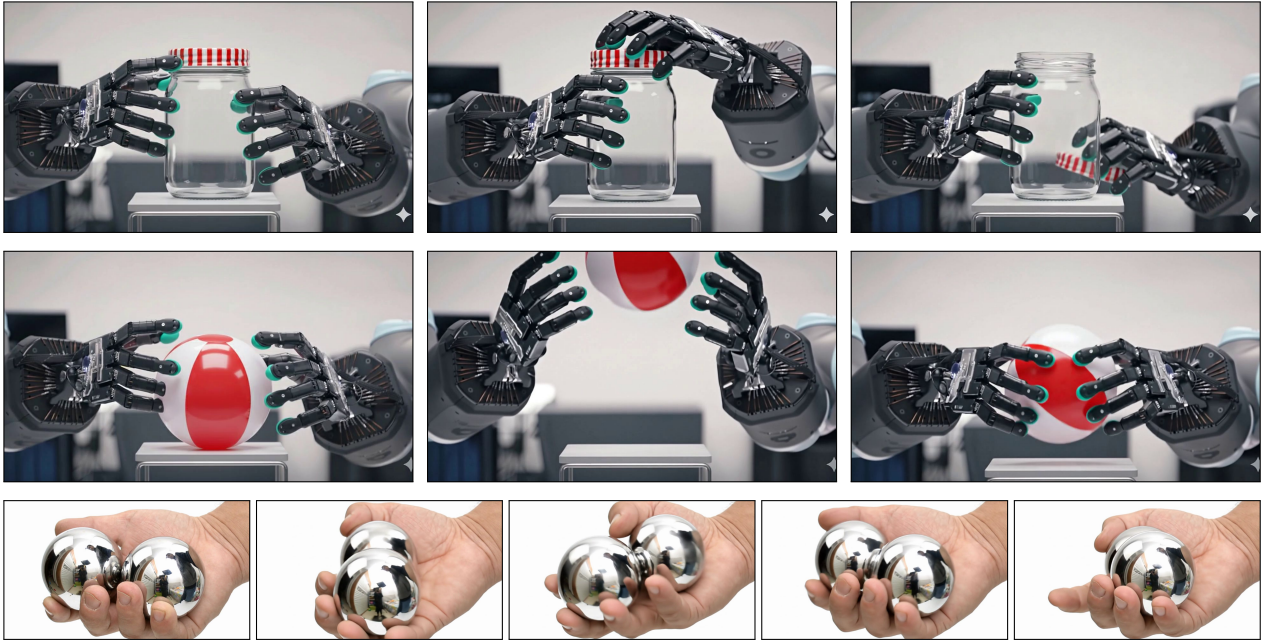
Figure 44 | Dexterous manipulation. Jar opening (top). Prompt: “Use common sense and have the two robot hands attached to robot arms open the jar, like how a human would.” Success rate: 1.0. Throwing and catching (middle). Prompt: “Use common sense and have the two robot hands attached to robot arms throw the ball in the air, the ball goes up off the screen, hands move to positions to catch the ball, and catch the falling ball, like how a human would.” Success rate: 1.0. Rotating Baoding balls (bottom). Prompt: “A human hand holds two metal Baoding balls. The fingers, including the thumb, index, and middle finger, skillfully manipulate the balls, causing them to rotate smoothly like two planets orbiting around each other and continuously in the palm, one ball circling the other in a fluid motion.” Success rate: 0.08.
